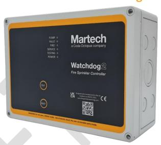
During normal operation Watchdog2 constantly monitors all inputs looking for changes in pressure or flow. A drop in pressure on any pressure switch will cause the pump to initially operate in jockey-mode to re-pressurise the system (i.e., for a slow leak) before switching to fire mode if pressure is not reinstated. Activation of the flow sensor at any time will trigger fire mode immediately.
