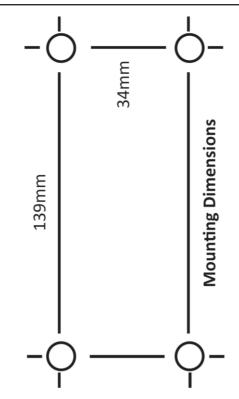
The Fire Sprinkler Watchdog should be fitted to a wall near the sprinkler pump. Fit the enclosure to the wall with the cable glands on the underside. The diagram above shows the positions for the four fixing screws. The fixing holes for the enclosure are revealed with the lid removed.
